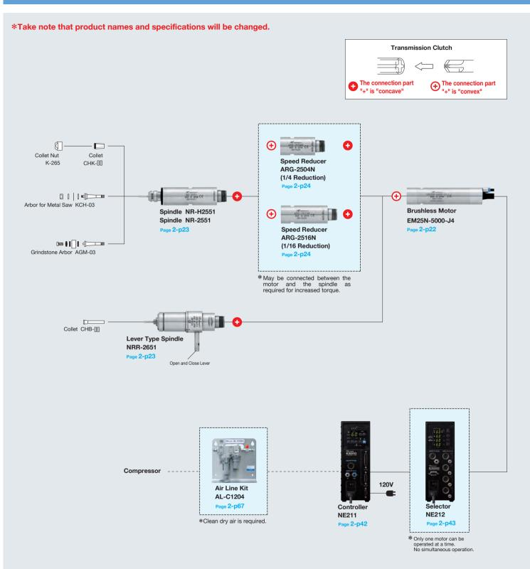
\* Do not exceed the maximum motor speed recommendation for the spindles. Excess speed will dramatically reduce bearing life.
